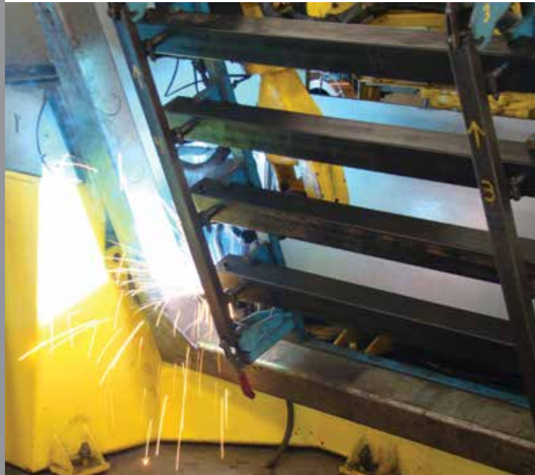
The metallic components are made of steel, welded and hot-dip galvanised.
